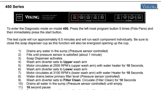
12) Dryer blower motor and heater will activate for **10** seconds to check amps When cycle is complete, you will hear 2 long Beeps. This is the indication that the test cycle has finished.
